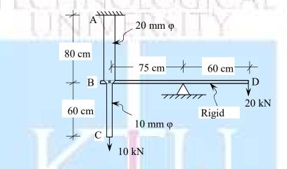
3. A rigid barABof length 100 cm, hinged at one end is supported by a steel rod and a copper wire as shown. Find the stresses induced in the rod and wire due to a downward load acting at 70 cm from the hinged end of the bar. Calculate the vertical deflection at B also. Modulus of elasticity of steel and copper are 200 GPa and 80 GPa respectively. Neglect the weight of the rigid bar.
