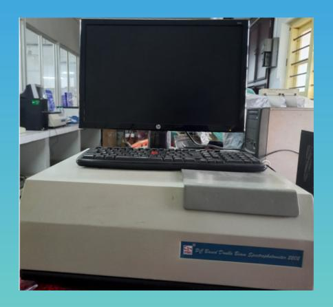
A double beam spectrophotometer is an instrument used to measure the absorption or reflection of light by a sample. It works by using two light sources, one reference beam and one test beam, and measuring their intensity before and after the sample, to calculate the amount of light absorbed by the sample.
