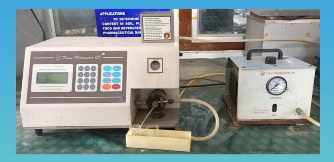
A flame photometer is an analytical instrument that measures the concentration of metal ions in a solution by emitting light of a specific wavelength. It is commonly used in clinical and environmental labs.
