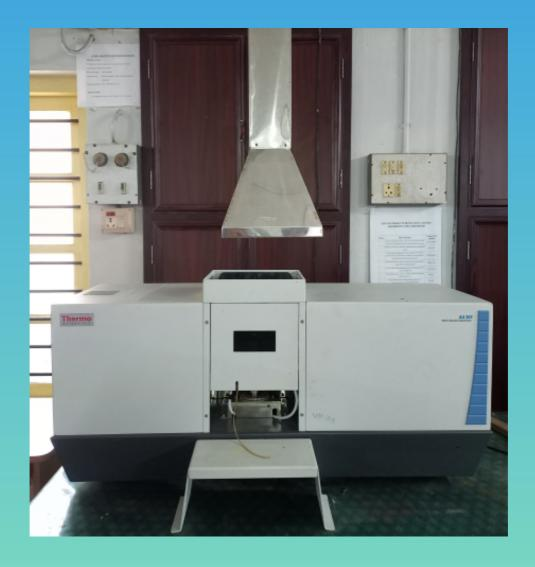
An atomic absorption spectrometer is a device used to measure the concentration of an element in a sample. It works by passing a beam of light through the sample and analyzing the intensity of the transmitted light for the presence of certain elements.
