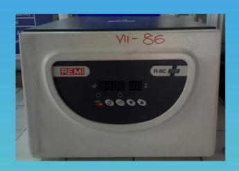
REMI laboratory centrifuge is a lab instrument that separates components based on their density by spinning samples at high speeds. It comes in various models and capacities.
